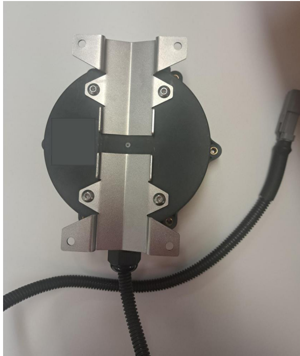
Figure 4. IntelliBlast Lite with mounting plates secured to the back of device
