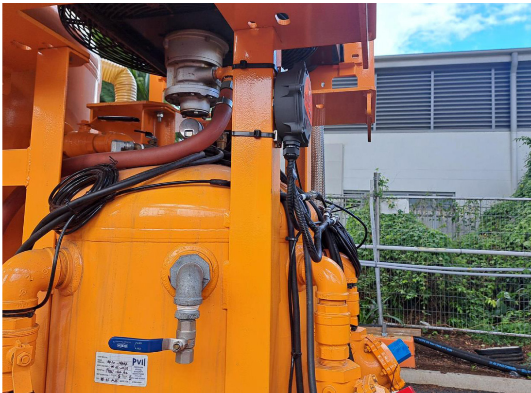
Figure 5. IntelliBlast Lite mounted to MEGA blast pot using zip-ties
