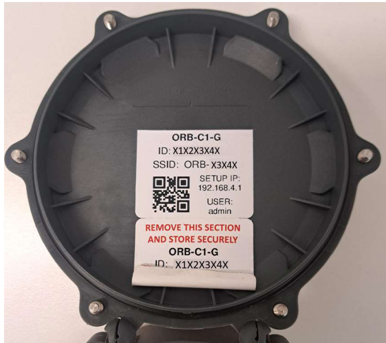
Figure 2. Device details found inside lid and unit (i.e. X1X2X3X4X)
